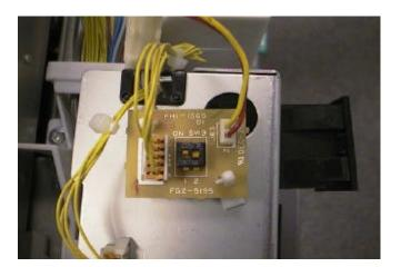
Refit control panel and covers and check operation of counter, large size copies or prints should now register on the option counter as well as the total counter.
